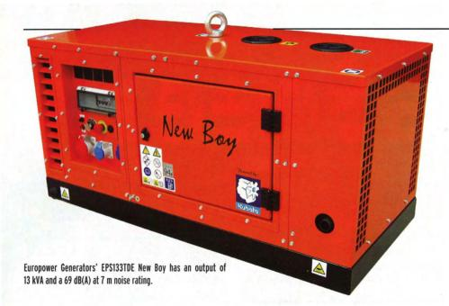
Europower Generators in Belgium has expanded its New Boy super-silenced line with the 13 kVA maximum output EPS133TDE model. Powered by a 14.5 kW Kubota engine, it is the same size - 138 x 64 x 68 mm - as the previously most powerful 11 kVA model. The 360 kg EPS133TDE has a noise level of 69 dB(A) at 7 m at 75% load, and it will run for 5.5 hours at full power on a tank of fuel.
